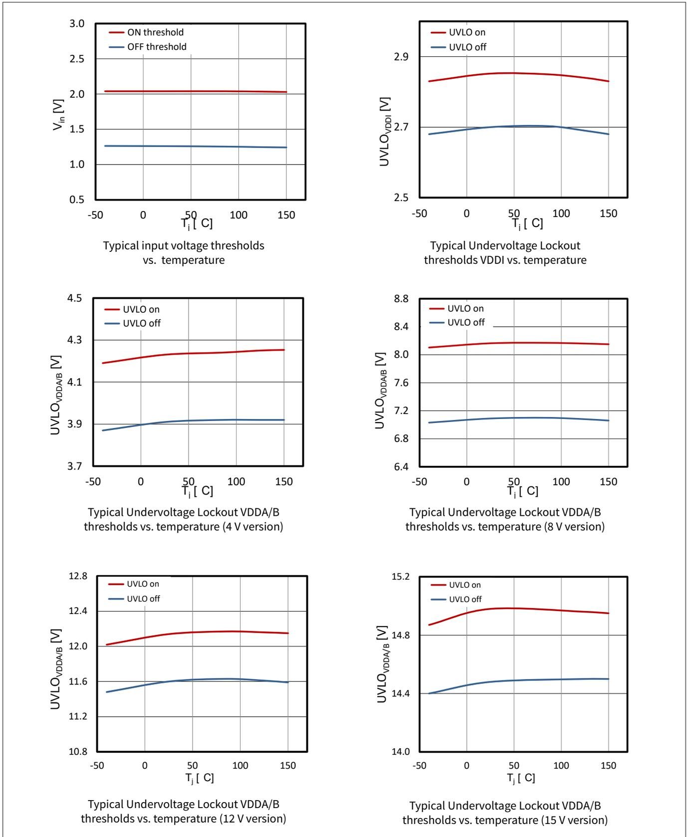
**Figure 17** Input voltage thresholds and Undervoltage Lockout
