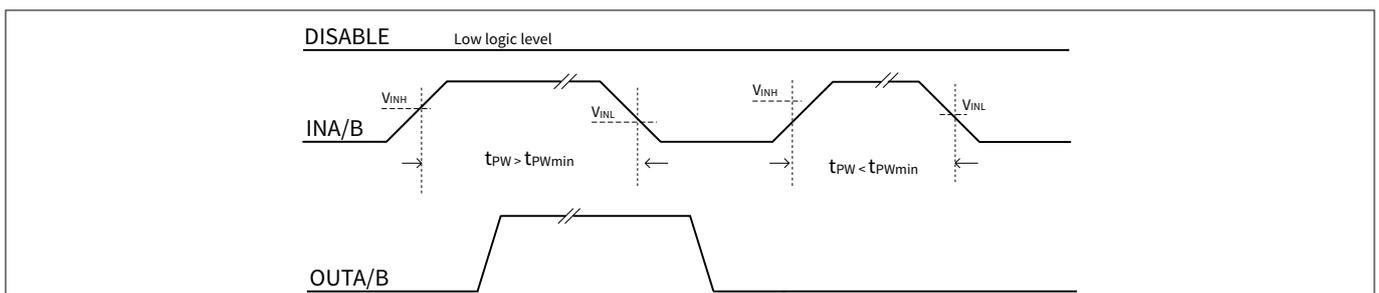
**Figure 11 Minimum pulse that changes the output state**
