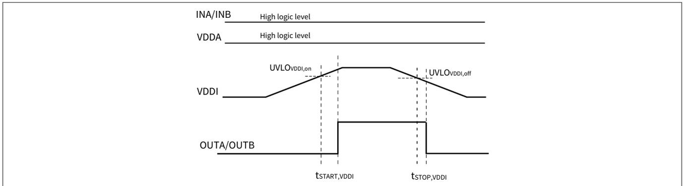
**Figure 12**  $V_{DDI}$  UVLO behavior, start-up and deactivation time
