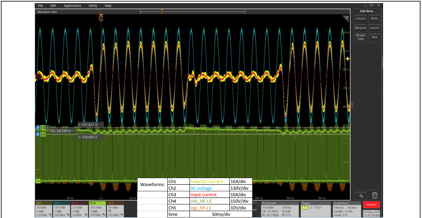
Figure 19 3.3 kW SiC totem-pole CCM PFC response for 10 percent to 90 percent load steps every 150 ms with 0.2 A/μs current slope
