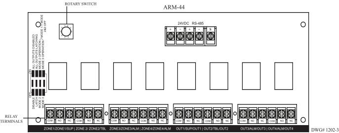
All field installed wiring connected to the panel and relay board must maintain a spacing of at least 1/4" between all electric light, power, class 1 or non-power limited fire protective signaling conductors.
