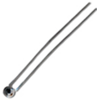
140 Series, 2,54 mm [0.1 in] disc thermistor with leads, 500 Ohm resistance, \pm 10.0\% tolerance, 25/85 BETA = 3468
