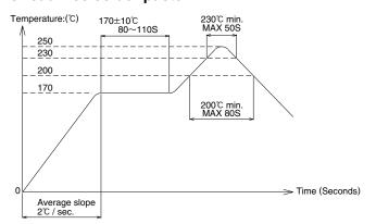
The temperature profile is based on the shown conditions. In individual applications the temperature may vary, depending on solder paste type, volume/ thickness and board size/thickness. Consult your solder paste and equipment manufacturer for specific recommendations.
