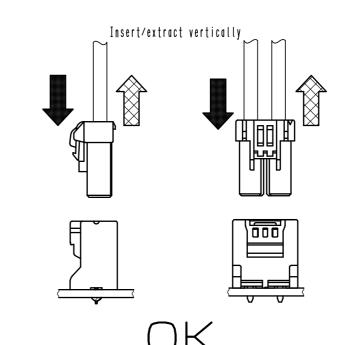
2) When it is hard to extract, please lightly insert the connector beforehand and then pull it with releasing the lock. Forced extraction has a risk of connector breakage.
