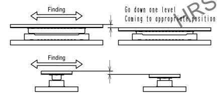
(2) When quiding, the connectors are aligned parallel to each other, with longitudinal and lateral movements restricted. Mate them properly by applying force in this condition.
