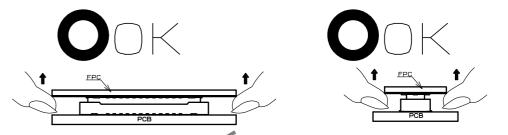
(2) If the connector common be un-mated parallel it can be removed diagonally from the pitch direction. Be careful to do so since this action applies stress on the contact.
