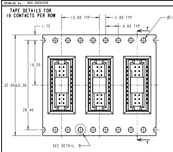
1.27 x (No. OF CONTACTS RECOMMENDED PCB LAYOUT Ø1.50<sup>+0.10</sup> TYP PER ROW - I) 1.27 TYP ->  $-0.50\pm0.05$ 7.40 SECTION Y-Y 0.70 TYP ->  $16.30\pm0.15$ 1.70<sup>+0.15</sup> TYP DETAIL B
