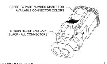
PLUG, 2 SOCKET, AT SERIES, STRAIN RELIEF END CAP
