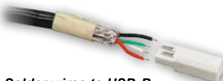
Solder wires to USB-B Insert
