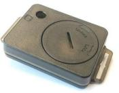
S-track Sense is a Bluetooth tag designed to record temperature, humidity and impact data. It uses BLE to transfer the information via beacon or mesh technology to the nearest gateway. A long battery life time and ruggedized enclosure (IP65) makes it suitable for cold chain monitoring. Easy programming and activation is enabled by NFC technology.
