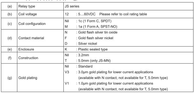
Note: Actual marking omits the hyphen (-). V3, V1 are marked at different position on the relay. E.g.: Ordering code: JS-12F actual marking: JS12F-K
