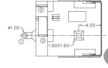
Recommended PCB Layout Top View
