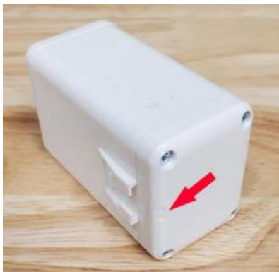
Figure 2-8 Proper Replacement Orientation of the Battery Cover
