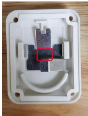
Figure 2-7 Polarity Marker and Battery Insertion
