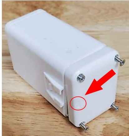
Figure 2-6 Removing the Battery Cover Screws
