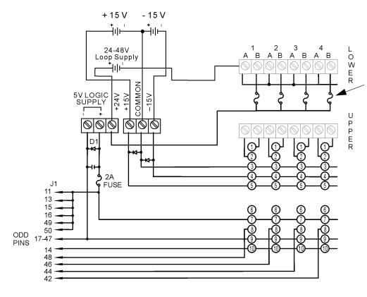
Install 1/8 amp fuse here to use the 24 VDC shared loop source. With fuse installed, shared loop source +24 VDC is available at lower B terminal. Fuses are provided with AD3, DA3, and DA8 modules.
