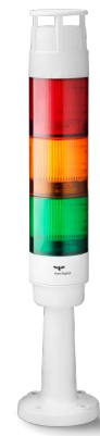
Order no.: CT5-Q06 Colours: red/amber/green Function: LED steady beacon, Piezo buzzer module, one of eight tones can be selected with a dip switch Nominal voltage: 24 V DC Type of mounting: Tube mounting (100 mm tube length)
