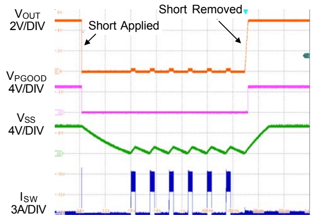
Figure 3. Short-Circuit Protection and Recovery
