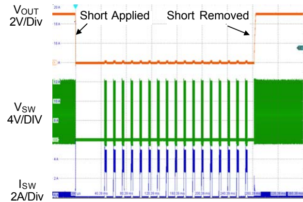
Figure 2. Short-Circuit Protection and Recovery
