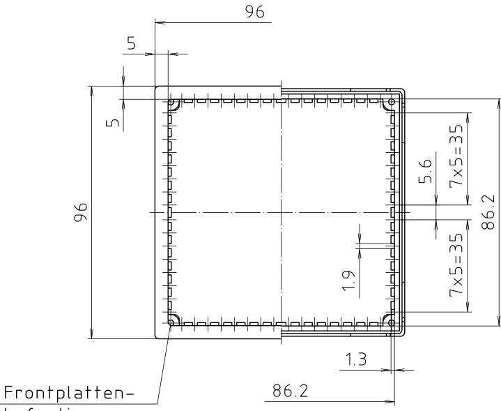
befestigung 84mm x 84mm/ front panel fixing points 84mm x 84mm
