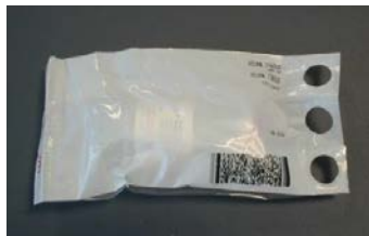
Figure 191. Overprinted Barcode Readable by ABR Through the Envelope Window Film
