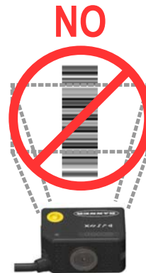
Figure 9. Code Out of FOV Due to Tilt Angle
