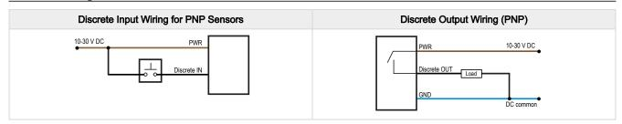
Connecting power to the communication pins will cause permanent damage. For the DX8x...C models, PWR in the wiring diagram refers to V+ on the wiring board and GND in the wiring diagram refers to V- on the wiring board. To power the sensor using the switch power output (SPx), replace the PWR with SPx in these wiring diagrams.
