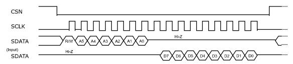
R/W : Instruction bit controls to write data to AK2365A or read back from it. When set to low, AK2365A is in write mode. When set to high, AK2365A is in read mode.
