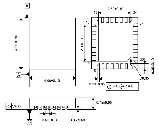
Note) The exposure pad(Exposed Pad) of the center of the package back is connected to opening or VSS.
