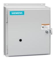
Electrically held lighting contactor, (convertible to mech. held), Amp rating 30A (tungsten 20A), 6 N.C. / 5 N.O. poles, 24V 60Hz / 20V 50Hz coil, Non-combination type, Encl NEMA type 4X 304 S-Steel, Water/dust tight noncorrosive
