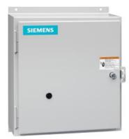
Electrically held lighting contactor, (convertible to mech. held), Amp rating 30A (tungsten 20A), 3 N.C. / 5 N.O. poles, 230-240V 60Hz/220V 50Hz coil, Noncombination type, Encl NEMA type 4X 304 S-Steel, Water/dust tight noncorrosive
