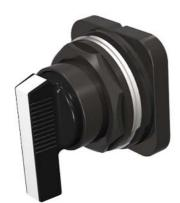
Selector switch, metal, NEMA 4X Spring return from left Long lever, B Cam 3 position Operator only white insert Non-Illuminated UL file E22655 in Vol. 6 (7) Sec. 13 (2)
