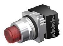
30mm Command/52, Chrome Finish Heavy Duty,Watertight/Oiltight Complete Metal Unit PTT / Illuminated Pushbutton Full Voltage, 6V AC LED Lamp Extended Button Plastic Lens, Red 2 Position Momentary with 1 N.O. - 1 N.C. Heavy Duty Contacts, A600/P600 UL Listed, CSA Certified NEMA 1,3,3R,4,4X,12,13 & Automotive Standards
