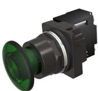
30mm BlackMax, Epoxy Coated Corrosion Resistant Complete Metal Unit Illuminated Push-Pull Operator Full Voltage, 24V AC/DC LED Lamp Mushroom Head Cap Small 1 3/4" (44.5 mm) Plastic, Green 3 Position Pull-Momentary/Push-Maintained UL Listed, CSA Certified NEMA 1,3,3R,4,4X,12,13 & Automotive Standards
