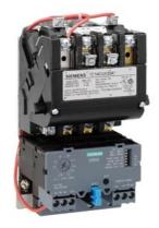
Non-reversing motor starter Size 0 Single phase full voltage Solid-state overload relay OLRelay amp range 3-12A 110-120/220-240VAC 60HZ coil Combination type No enclosure
