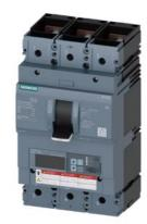
circuit breaker 3VA6 UL frame 600 breaking capacity class H 65kA @ 480 V 3pole, line protection ETU550, LSI, In=600A overload protection Ir=240A ...600A short-circuit protection Isd=0.6..9x In, Ii=1.5..9x In N conductor protection opt. w. ext. CT; up to 160% nut keeper kit on both sides
