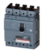
circuit breaker 3VA6 UL frame 600 breaking capacity class C 100kA @ 480V 4pole, line protection ETU856, LSI, In=400A overload protection Ir=160A...400A short-circuit protection Isd=0.6..10x In, Ii=1.5..12x In N conductor protection adjustable (OFF, up to 160%) ground-fault alarm message via EFB300 or COM without connection
