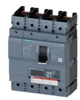
circuit breaker 3VA6 UL frame 600 breaking capacity class C 100kA @ 480V 4-pole, line protection ETU860, LSIG, In=400A overload protection Ir=160A...400A short-circuit protection Isd=0.6..10x In, Ii=1.5..12x In N conductor protection adjustable (OFF, up to 160%) ground-fault protection Ig=0.2...1 x In= tg=0.05-0.8s without connection
