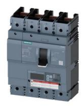
circuit breaker 3VA6 UL frame 600 breaking capacity class C 100kA @ 480V 4-pole, line protection ETU556, LSI, ln=400A overload protection lr=160A...400A short-circuit protection lsd=0.6..10x ln, li=1.5..12x ln N conductor protection adjustable (OFF, up to 160%) ground-fault alarm message via EFB300 or COM without connection
