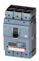
circuit breaker 3VA6 UL frame 600 breaking capacity class C 100kA @ 480 V 3-pole, line protection ETU556, LSI, In=400A overload protection Ir=160A ...400A short-circuit protection Isd=0.6..10x In, Ii=1.5..12x In N conductor protection opt. w. ext. CT; up to 160% ground-fault alarm message via EFB300 or COM cable connection on both sides
