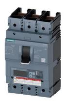
circuit breaker 3VA6 UL frame 600 breaking capacity class C 100kA @ 480V 3-pole, line protection ETU560, LSIG, In=400A overload protection Ir=160A...400A short-circuit protection Isd=0.6..10x In, Ii=1.5..12x In N conductor protection optionally with external current transformer, up to 160% ground-fault protection Ig=0.2...1 x In, tg=0.05-0.8s without connection
