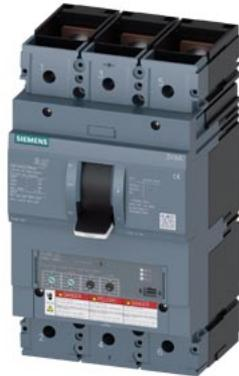
Circuit breaker 3VA6 UL Frame 600 breaking capacity class C 100kA @ 480 V 3-pole, Line protection ETU330, LIG, In=400A overload protection, 100% rated Ir=160A ...400A Short-circuit protection Ii=1.5...12 x In Ground-fault protection Ig=0.2... 1 x In, tg=0.1/0.3s nut keeper kit on both sides
