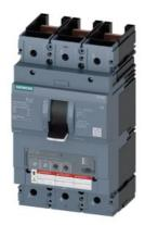
circuit breaker 3VA6 UL frame 600 breaking capacity class C 100kA @ 480V 3-pole, line protection ETU330, LIG, ln=400A overload protection Ir=160A...400A short-circuit protection li=1.5...12 x ln ground-fault protection lg=0.2...1 x ln, tg=0.1/0.3s without connection
