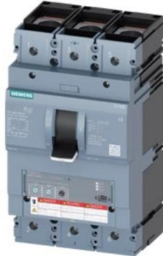
Circuit breaker 3VA6 UL Frame 600 breaking capacity class C 100kA @ 480 V 3-pole, Line protection ETU320, LI, In=400A overload protection, 100% rated Ir=160A ...400A Short-circuit protection Ii=1.5...12 x In cable connection on both sides
