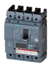
Circuit breaker 3VA6 UL frame 250 breaking capacity class M 35kA @ 480V 4-pole, Line protection ETU830, LIG, In=250A overload protection, 100% rated Ir=100A...250A Short-circuit protection Ii=1.5...10 x In Ground-fault protection Ig=0.2...1 x In, tg=0.05-0.8s without connection
