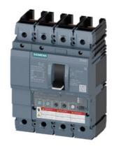
Circuit breaker 3VA6 UL frame 250 breaking capacity class M 35kA @ 480V 4-pole, Line protection ETU350, LSI, In=100A overload protection, 100% rated Ir=40A...100A Short-circuit protection Isd=1.5...10 x Ir, Ii=12 x In N conductor protection adjustable (OFF, 50%, 100%) without connection
