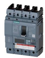
Circuit breaker 3VA6 UL Frame 150 breaking capacity class C 100kA @ 480V 4pole, Line protection ETU860, LSIG, In=40A overload protection, 100% rated Ir=16A...40A Short-circuit protection Isd=0.6..10x In, Ii=1.5..12x In N conductor protection adjustable (OFF, up to 160%) Ground-fault protection Ig=0.375...1 x In= tg=0.05-0.8s without connection
