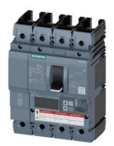
circuit breaker 3VA6 UL frame 150 breaking capacity class H 65kA @ 480V 4-pole, line protection ETU830, LIG, In=100A overload protection Ir=40A...100A short-circuit protection Ii=1.5...12 x In ground-fault protection Ig=0.2...1 x In, tg=0.05-0.8s without connection
