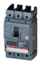
Circuit breaker 3VA6 UL Frame 150 breaking capacity class H 65kA @ 480V 3-pole, Line protection ETU820, LI, In=100A overload protection, 100% rated Ir=40A...100A Short-circuit protection Ii=1.5...12 x In without connection
