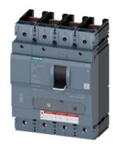
CIRCUIT BREAKER 3VA5 UL Frame 400 BREAKING CAPACITY CLASS H 65kA @ 480 V 4POLE, LINE PROTECTION TM240, ATAM, In=400A OVERLOAD PROTECTION IR=280A ...400A SHORT CIRCUIT PROTECTION II=5...10 x In NEUTRAL UNPROTECTED W/O CONNECTION
