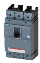
MOLDED CASE SWITCH 3VA5 UL FRAME 400 MAX SHORT CIRCUIT CURR. RATING 65kA @ 480 V 2POLE, LINE PROTECTION MCS110, In=400A WITHOUT OVERLOAD PROTECTION SELF PROTECTION II=15 x In W/O CONNECTION
