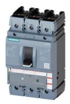
circuit breaker 3VA5 UL frame 250 breaking capacity class H 65kA @ 480 V 3-pole, line protection TM240, ATAM, In=250A overload protection Ir=200A ...250A short-circuit protection li=5...10 x In cable connection on both sides
