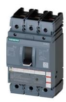
circuit breaker 3VA5 UL frame 250 breaking capacity class H 65kA @ 480 V 3-pole, line protection TM210, FTFM, In=250A overload protection Ir=250A fixed short-circuit protection Ii=10 x In nut keeper kit on both sides
