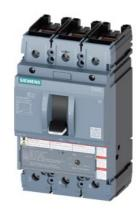
circuit breaker 3VA5 UL frame 250 breaking capacity class H 65kA @ 480 V 3-pole, line protection TM230, FTAM, In=250A overload protection Ir=250A fixed short-circuit protection Ii=5...10 x In UL489 SB (naval), 50 deg. cel. cable connection on both sides
