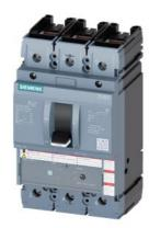
circuit breaker 3VA5 UL frame 250 breaking capacity class C 100kA @ 480 V 3-pole, line protection TM240, ATAM, In=150A overload protection Ir=120A ...150A short-circuit protection Ii=5...10 x In cable connection on both sides
