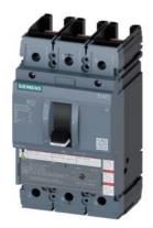
circuit breaker 3VA5 UL frame 250 breaking capacity class C 100kA @ 480V 3-pole, line protection TM210, FTFM, In=150A overload protection Ir=150A fixed short-circuit protection Ii=10 x In UL 489 SB (naval), 50° C without connection
