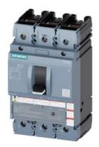
circuit breaker 3VA5 UL frame 250 breaking capacity class H 65kA @ 480 V 3-pole, line protection TM210, FTFM, In=150A overload protection Ir=150A fixed short-circuit protection Ii=10 x In UL489 SB (naval), 50 deg. cel. cable connection on both sides
